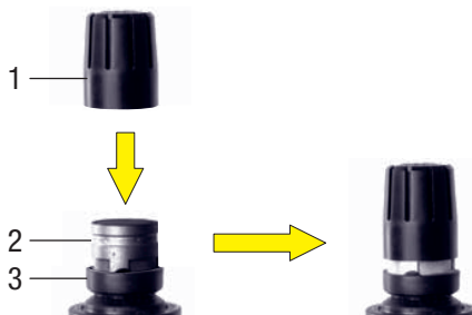
Figura 6: Instalar o PPC1000/PB1000
